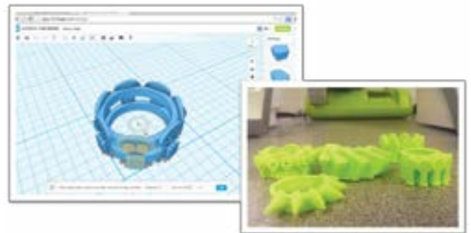
Figure 6. Screenshot of a digital model ring design in Autodesk 123d Design (left) and photograph of 3D printed rings (right).
